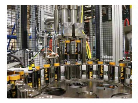
Martin Specialty Products' patented shrink sleeving of lubricating grease tubes and tubs has established a new benchmark in the finished production of lubricating greases. Shrink sleeving has solved many issues seen with the usage of traditional fiber tubes and plastic tubes including bleed through, leakage, and low-quality graphics. Shrink sleeving lubricating grease tubes and tubs produces a seamless, eye-catching product that drives consumer interest on the shelf.
