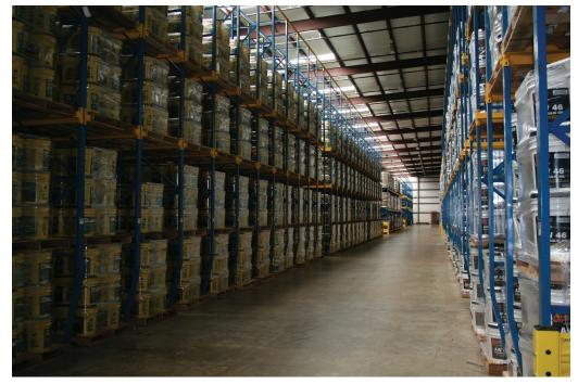
possible moisture contamination. A temperature range of 0°F and 110°F is acceptable for storage of most lubricants and greases. Ideally, the storage temperature range should be 32°F to 77°F.
